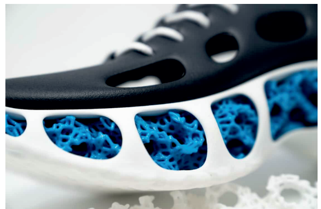
In a seamlessly integrated end-to-end value chain for industrial additive manufacturing this midsole was printed
