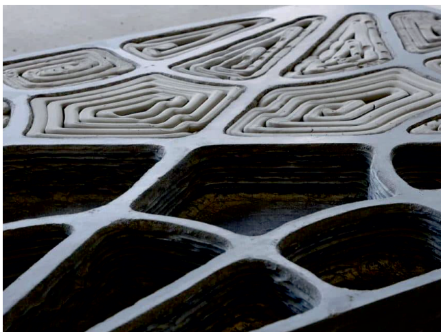
Ultra high-performance fibre-reinforced concrete is poured around the formwork elements
