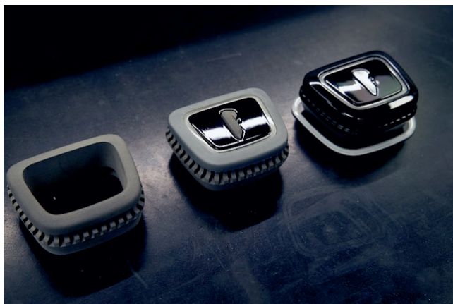
Multi-material combinations realized via multiple 3D-printing formats.
