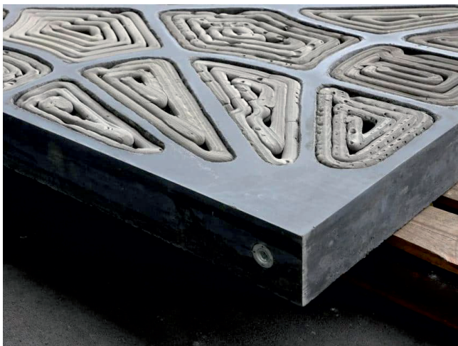
The FoamWork provides additional insulation through its porosity
