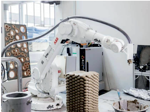
The system was 3D-printed using an autonomous robotic arm
