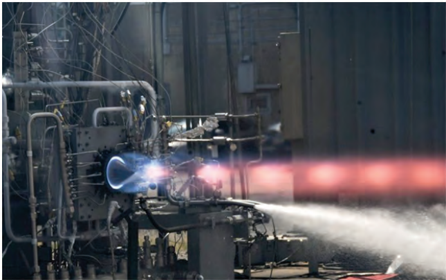
Rotating detonation rocket engine, or RDRE hot fire test at Marshall Space Flight Center. Credits: NASA
