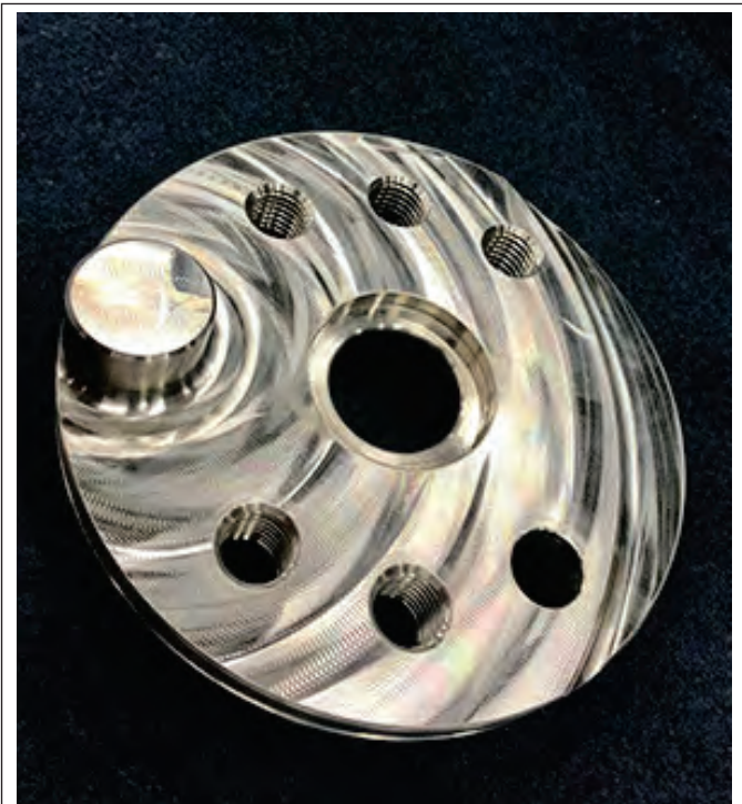
the crank disk 3D printed by Aidro with EOS M290 and machined by Kongsberg
