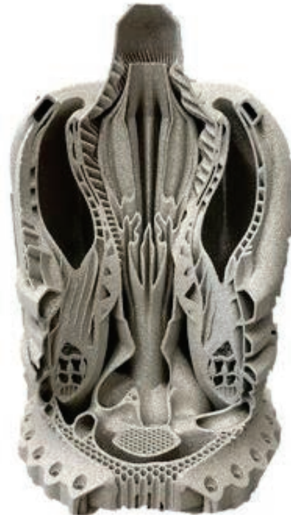
The futuristic Aerospike designed by Hyperganic. This part is 3D printed at TII using the Ni super alloy (IN718) and is considered the most complex 3D printed component ever among the AM community.
