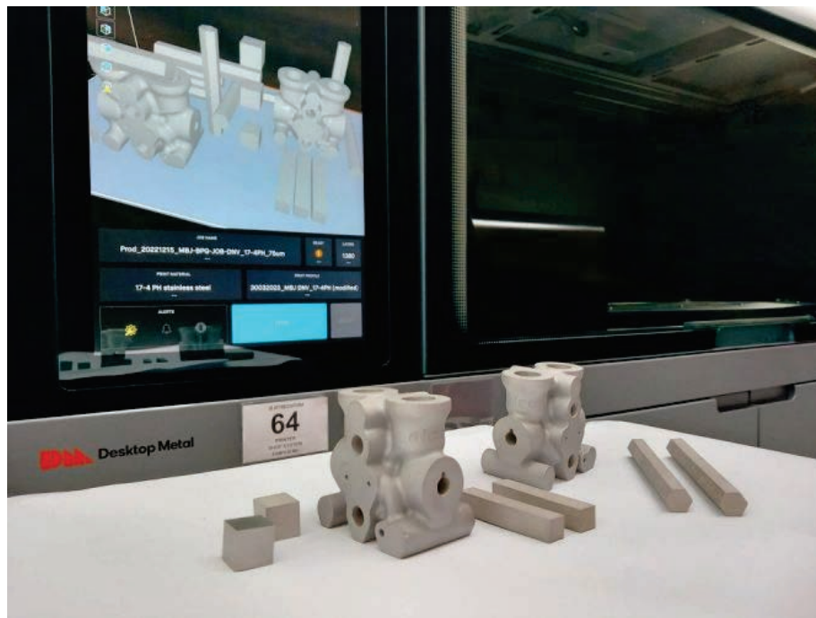
Aidro received the industry's first certification of qualification from DNV for binder jetting using the Desktop Metal Shop System™ for 3D printing 17-4PH stainless steel parts. The printer is shown here with two valves and coupons printed in 17-4PH. (Photo: Business Wire)
