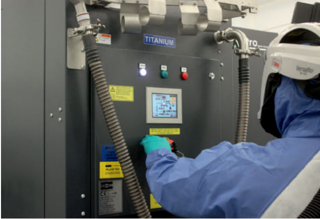
Figure 3. A key feature of the Russell AMPro® Sieve Station is its one-button automation system, which allows the operator to concentrate on other important value-added tasks.
