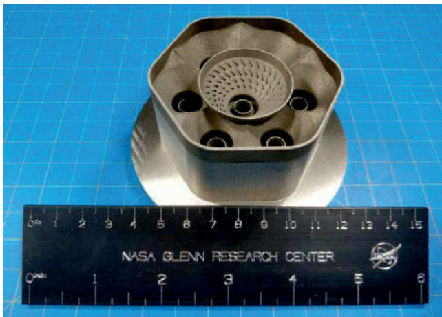
This turbine engine combustor (fuel-air mixer) was 3D-printed at NASA Glenn and is one example of a challenging component that can benefit from applying the new GRX-810 alloys.
