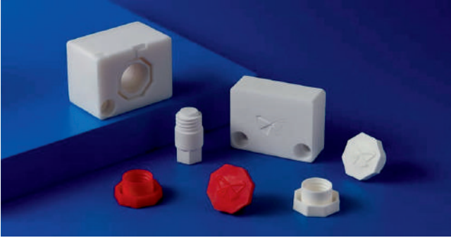
The printed three-part mould with the caps injected in polyethylene
