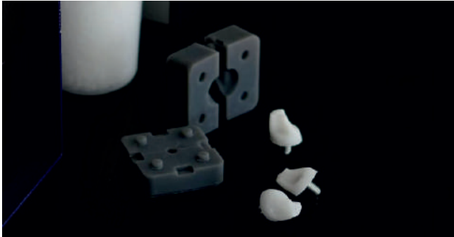
POM football cleats injected in the Holipress from moulds printed with Grey Pro Resin.
