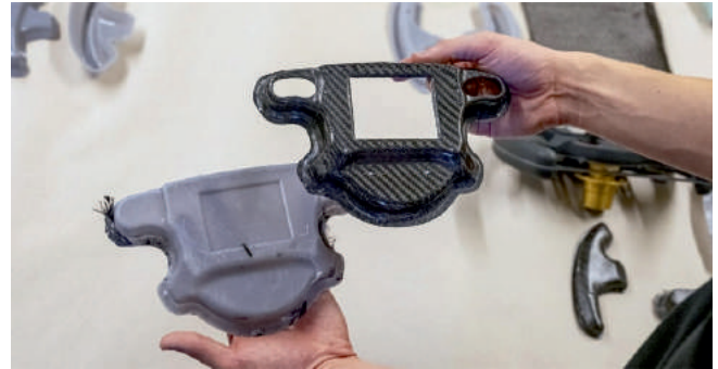
The 3D printed mould and the demoulded carbon fiber part for the steering wheel front housing.
