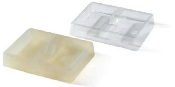
A vacuum forming mould printed in Formlabs High Temp Resin accompanied by the final vacuum formed part.
