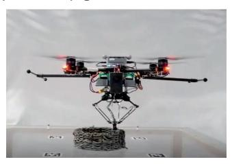
Researchers have created a team of drones that can 3d print while they are flying. These flying robots can coordinate and make decisions about how to print objects that are bigger than themselves – expanding the horizons of the construction industry.
