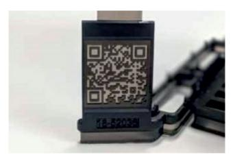
Custom QR codes and other tracking features can be directly incorporated into the part design without generating any additional process steps.
