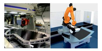
Figure 2: ATL/AFP head (a)gantry type (b) robot with AFP Head laying onto a female tool
