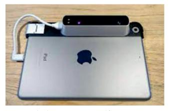
Figure 3: IPad with Structure Sensor used for scanning
