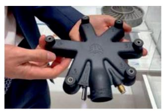
Assembly features can be directly incorporated into the component design.
