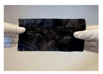
Researchers in the Lyding Group at the University of Illinois Urbana-Champaign discovered an efficient, sustainable method for 3D-printing single-walled carbon nanotube films, or thin aggregated sheets of carbon nanotubes that are adaptive enough to outfit an aircraft or contour to the human body.
