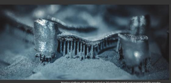
Printing platform with object printed on 3d printer for metal and covered metallic powder
