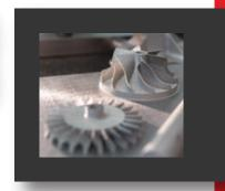
then fusing these layers together with a laser.
