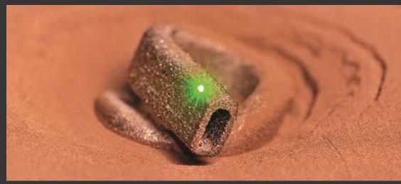
Green Laser on Copper Powder Bed. (Credit: Fraunhofer Institute, Germany)
