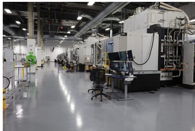
VulcanForms' new facility homes a fleet of 100kW laser 3d printing programs. Picture by way of VulcanForms.
