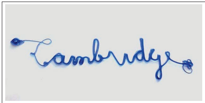
A 3D-printed cursive “Cambridge” printed using reinforcement learning. Credit: Soft Math Lab/Harvard SEAS
